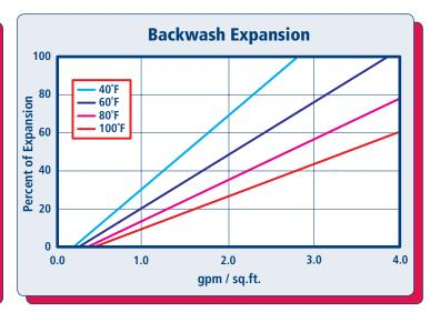
The graph above shows the expansion characteristics of ResinTech MBD-10 as a function of flow rate at various temperatures.
